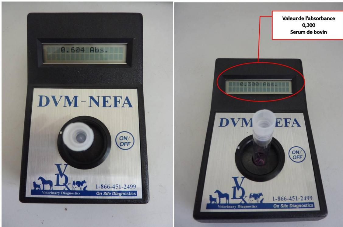
FIGURE 21 EXEMPLE DE MESURE DE L'ABSORBANCE AVEC LE DVM NEFA TEST SUR LA SOLUTION DONT LA CONCENTRATION EST CONNUE (PHOTO A GAUCHE) ET SUR UN DES ECHANTILLONS (PHOTO A DROITE) (G. FORGEAT)
